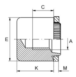
Female thread A = M3Height K = 9.0Min thread length C = 3.0Outer diameter E = 8.0Plate thickness = 2.6 to 2.8
